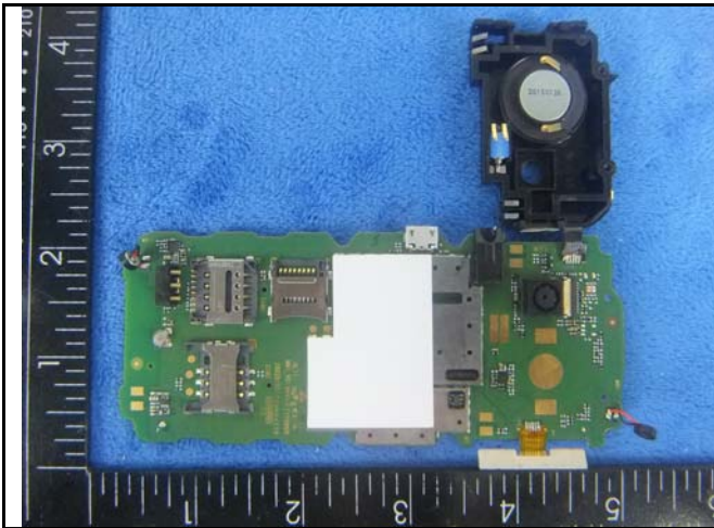
Mainboard With Shielding - Front View
