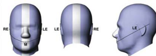
Figure 6.2 Front, back and side view of SAM
