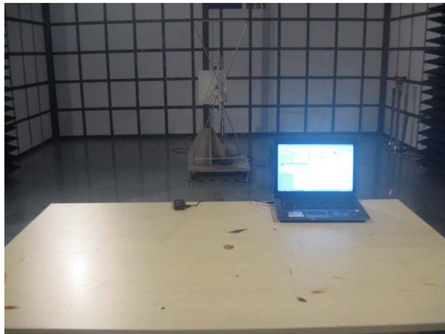
**Radiation Emission Test Setup (9kHz to 30MHz)**
