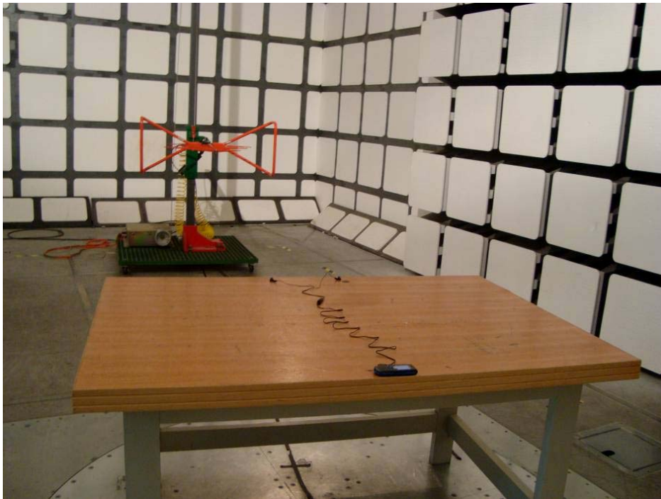
Radiated Emissions - Rear View (Media Playing mode)
