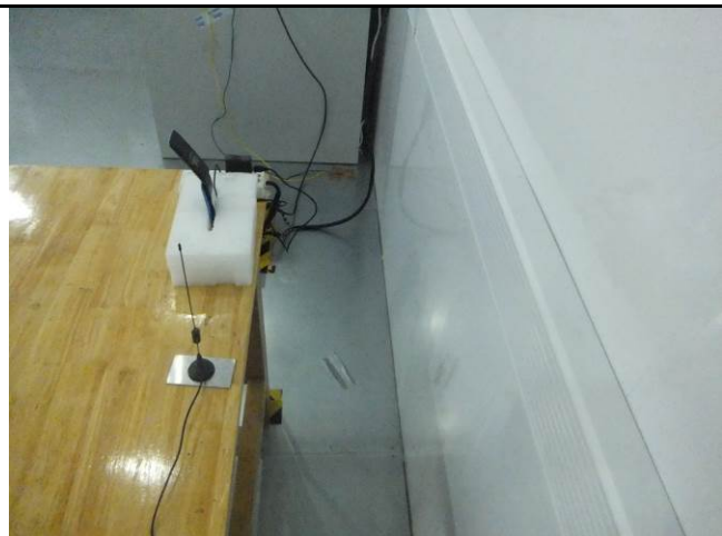
Conducted Emissions Test Setup Side View
