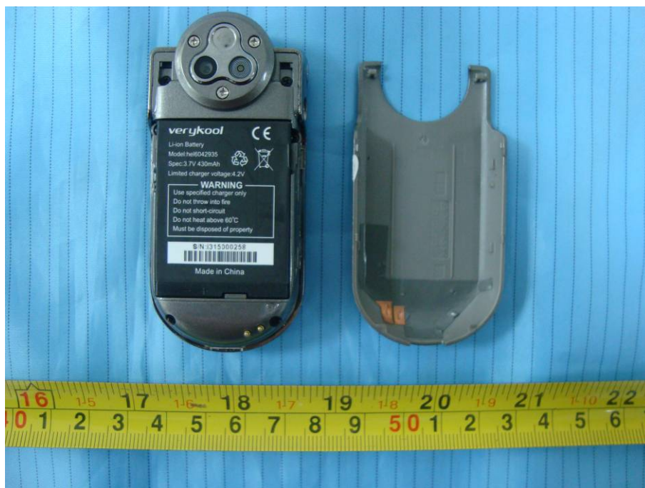
EUT – Cover off View 1
