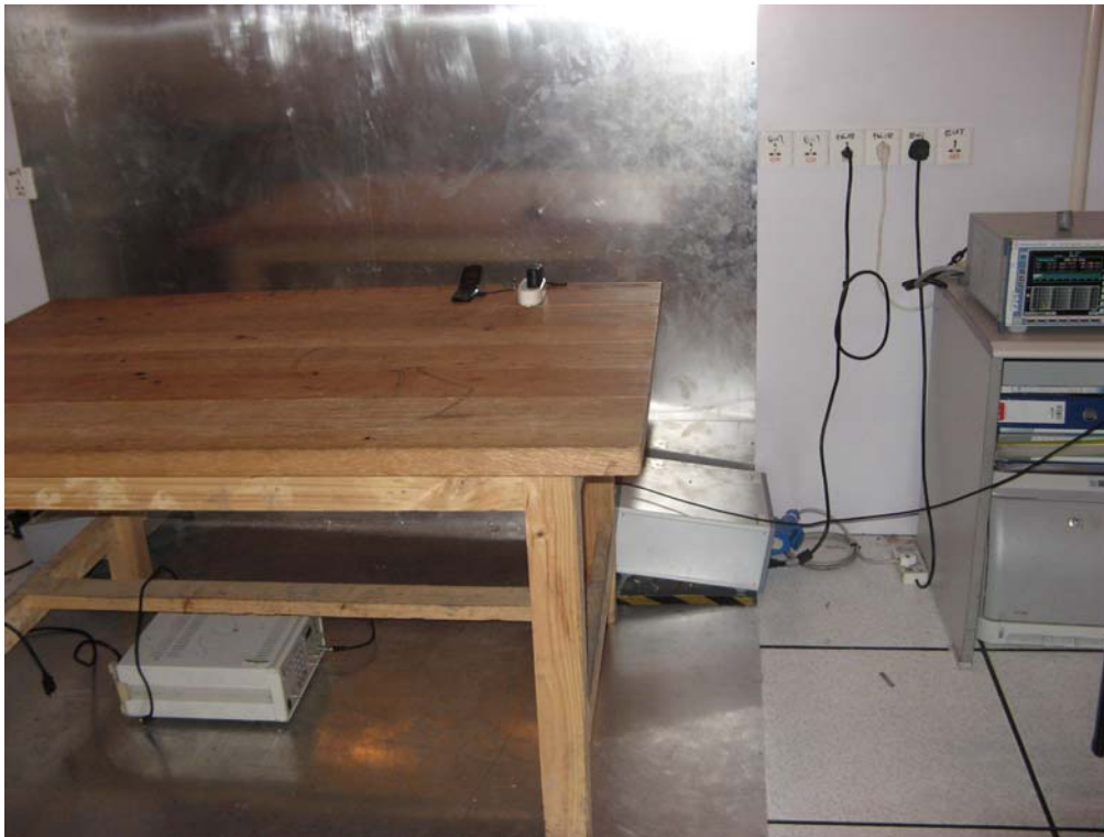
Conducted Emission Test Setup
