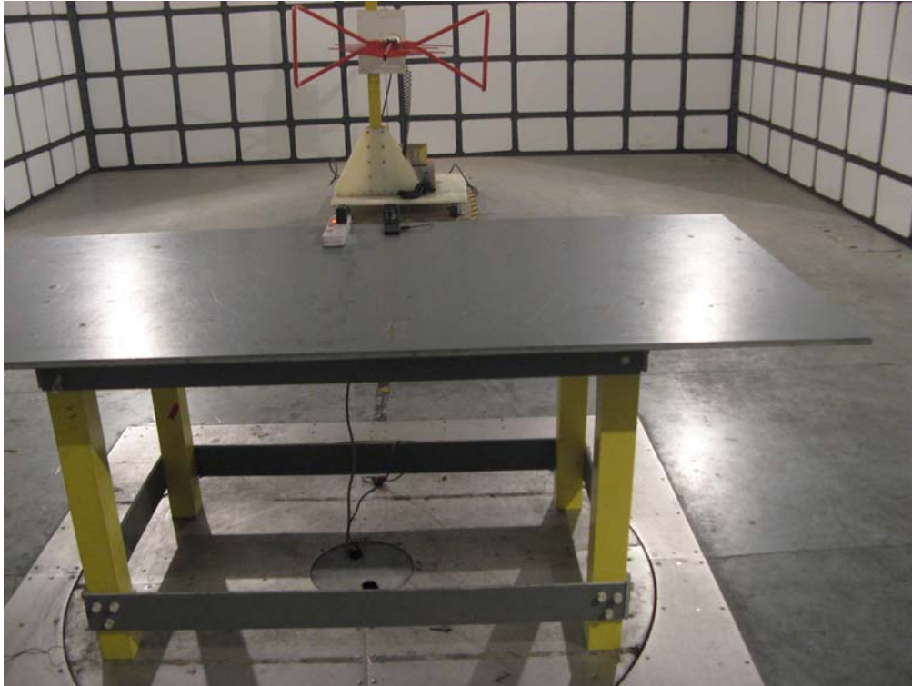
Radiated Emission Test Setup
