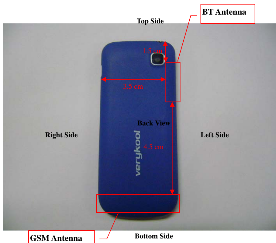
Fig 7.5 Block Diagram for EUT Antenna Position
