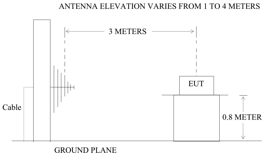
(EUT: Wireless weather station (Transmitter))
