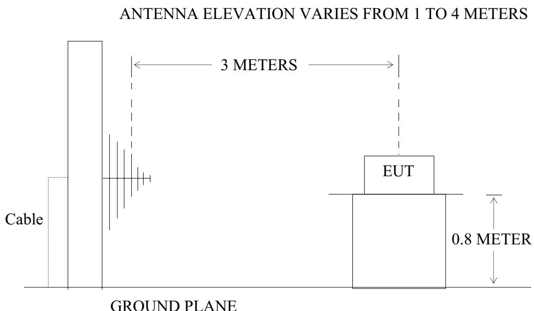
(EUT: Wireless weather station (Transmitter))
