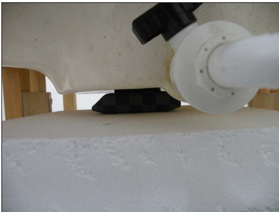
< Body SAR setup with holster-2 >
