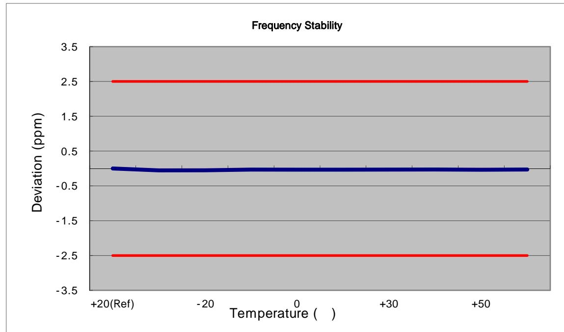
**7.7.2 FREQUENCY STABILITY (GSM1900)**OPERATING FREQUENCY: 1880,000,000 HzCHANNEL: 661REFERENCE VOLTAGE: 12.0 VDCDEVIATION LIMIT: -
