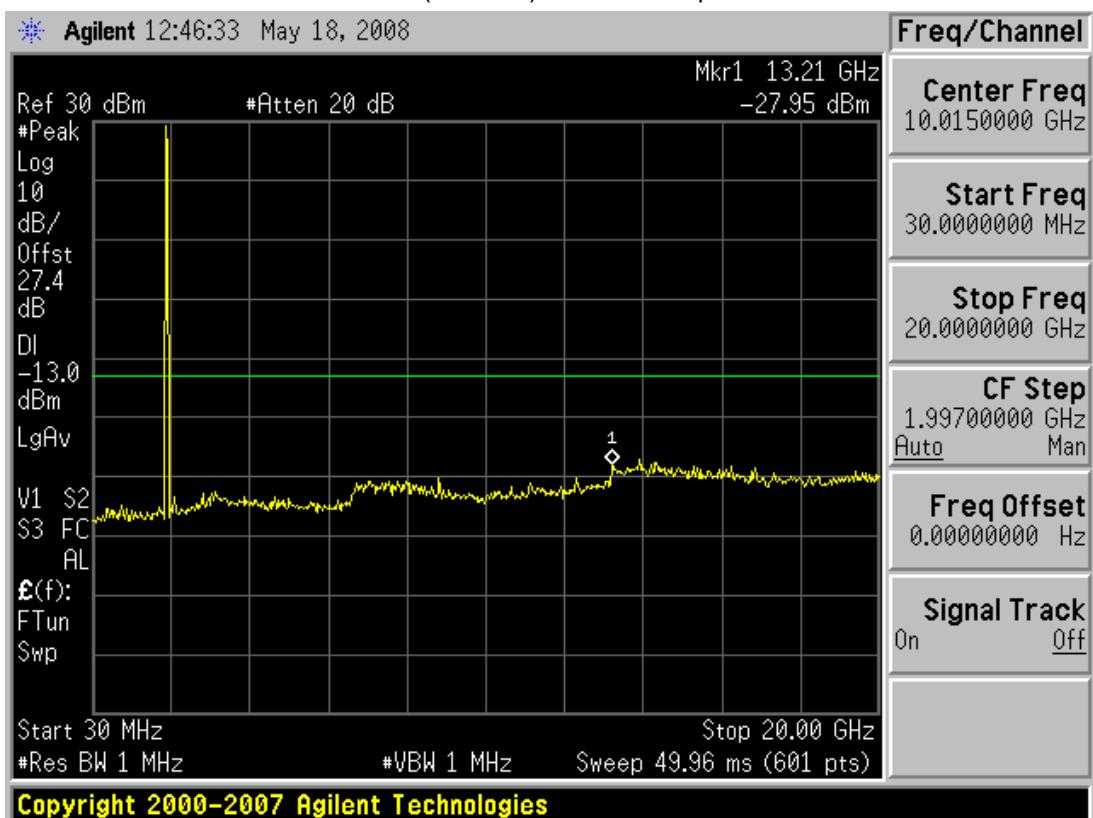
■ GSM1900 MODE (661 CH.) Conducted Spurious Emissions
