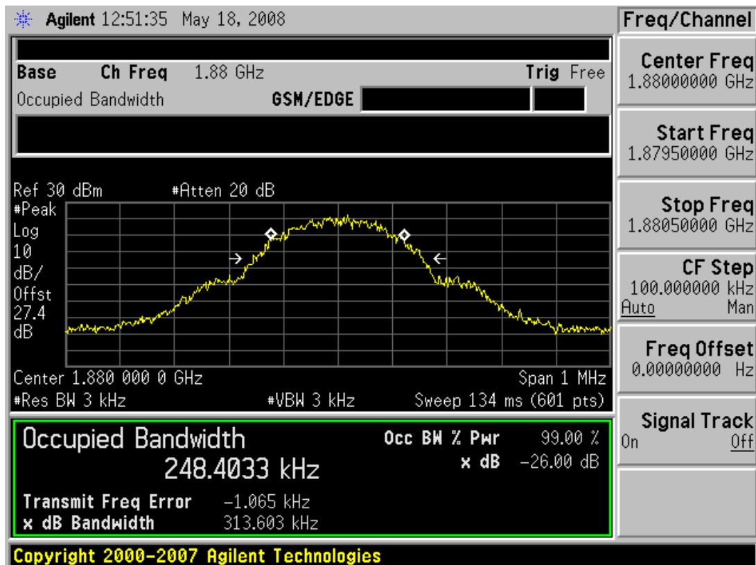
■ GSM1900 MODE (810 CH.) Occupied Bandwidth
