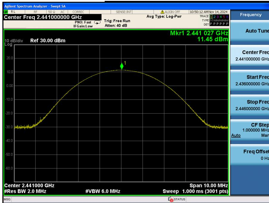
**Peak Output Power****Highest Channel & Modulation : 8DPSK**
