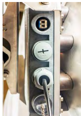
2 Unscrew the cap of the SFP port (LAN2 or LAN3) that will be used and install a SFP module.
