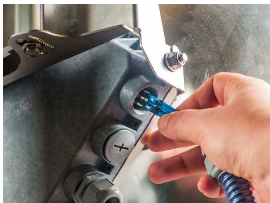
5 Connect LC connector to SFP module.
