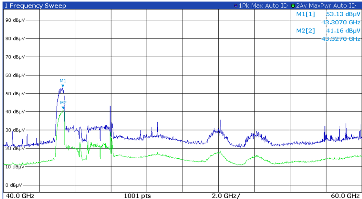
Figure 4.1 Radiated Spurious Emissions 40 – 60 GHz (Horizontal)
