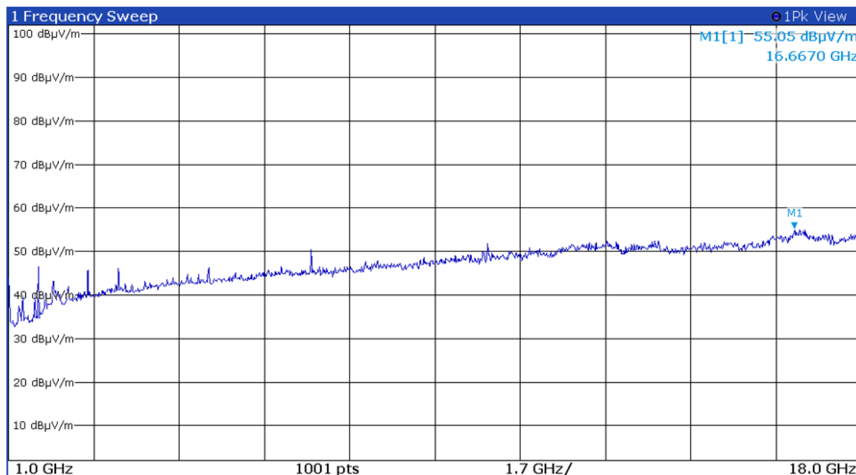
Figure 5.1 Radiated Spurious Emissions 1 – 18 GHz (Horizontal)
