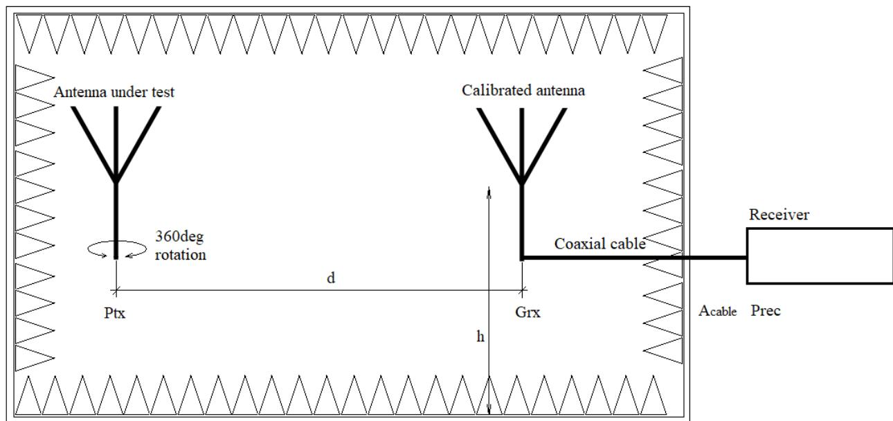
Gain of antenna under test is calculated as follows:
