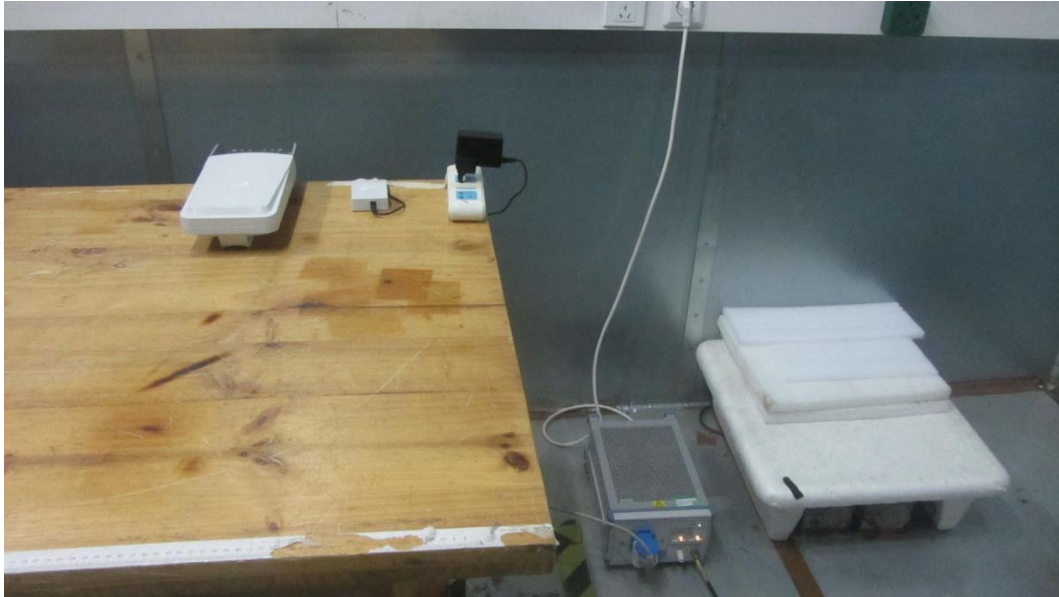
Picture 3 Conducted Emission Test Setup
