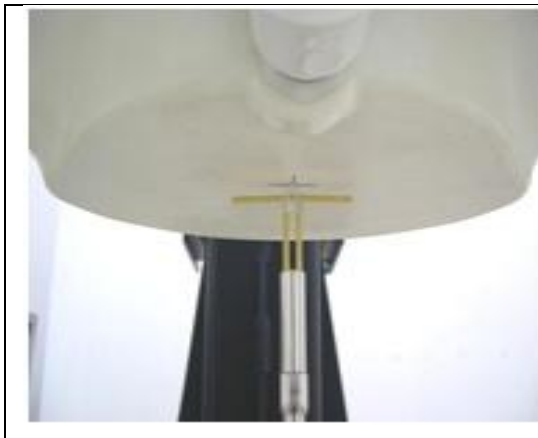
Fig 7.1 Photo of Dipole Setup
