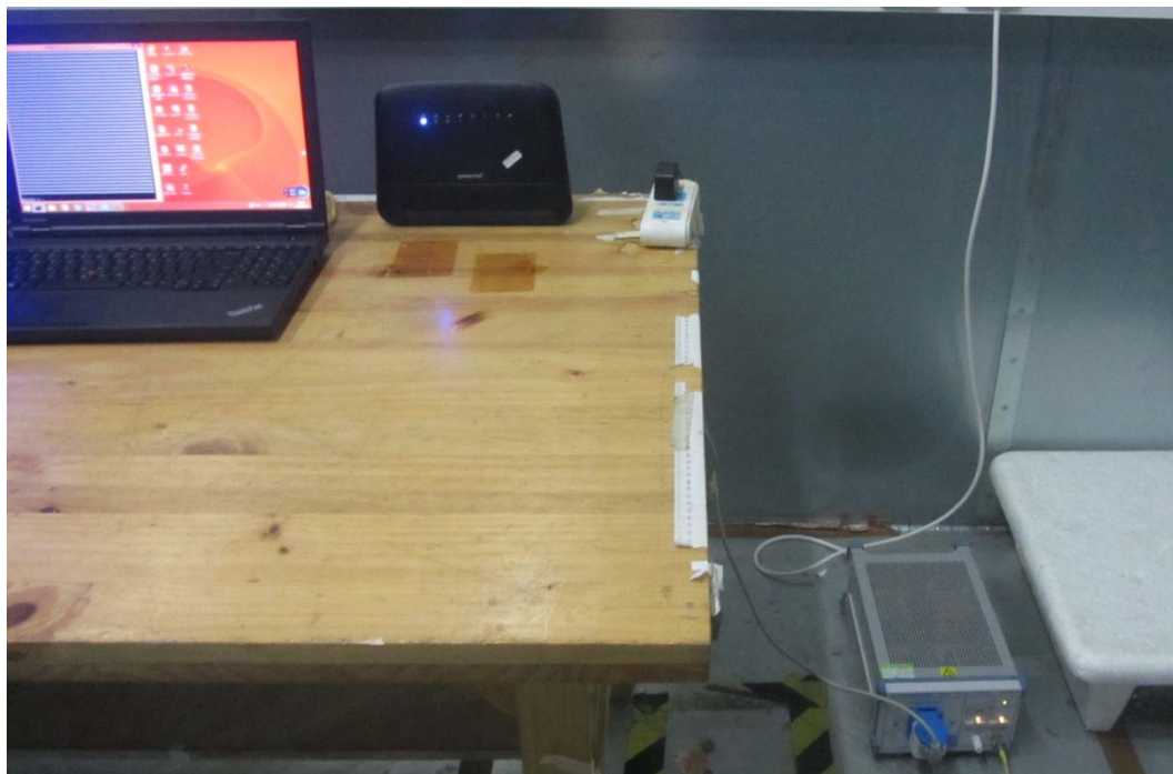
Picture 3 Conducted Emission Test Setup
