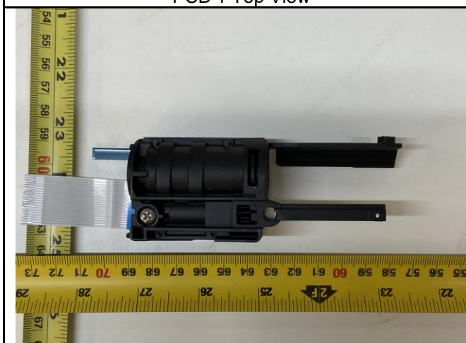
Internal Enclosure inside Key Box Containing Motor Gear Assembly and Main Circuit Board
