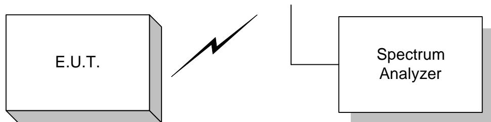
**Outdoor Test Site For Radiated Emissions****Radiated Emissions 30 MHz – 26.5 GHz**
