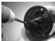
2. Remove the screws from the lid and open the call bell's case.
