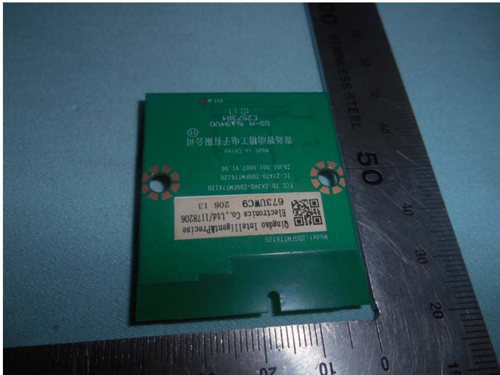
FIGURE 13 LED LCD TV (M/N: 55H6D) RF BOARD (SOLDERED SIDE)
