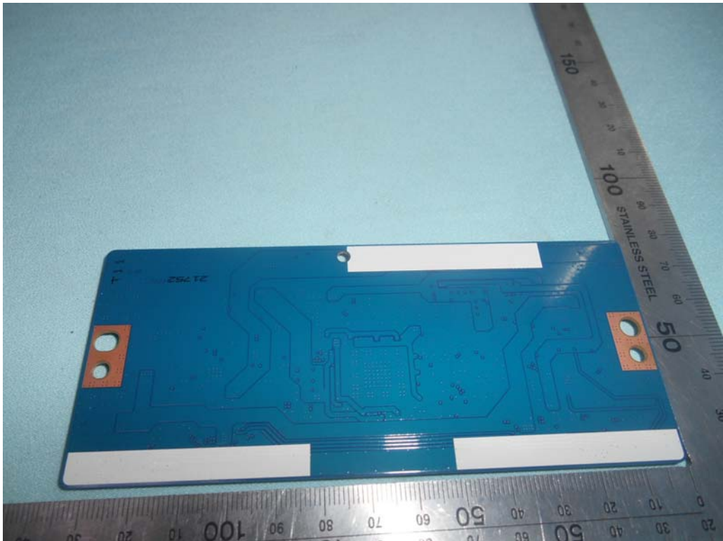
FIGURE 10 LED LCD TV (M/N: 55H6D) PANEL CONTROL BOARD (SOLDERED SIDE)
