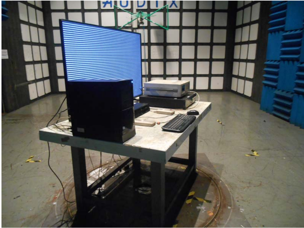
SETUP WITH MAXIMUM DETECTED EMISSION AT HORIZONTAL POLARIZATION (TEST MODE: HDMI 1024*768@60Hz & 1kHz PLAYING)
