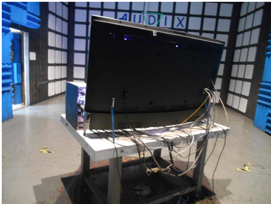
SETUP WITH MAXIMUM DETECTED EMISSION AT VERTICAL POLARIZATION (TEST MODE: HDMI 1920*1080@60HZ & 1KHZ PLAYING)
