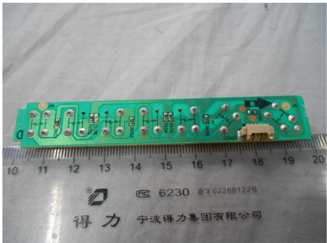
FIGURE 12 LED LCD TV (M/N: 55H4G) KEY BOARD (SOLDERED SIDE)
