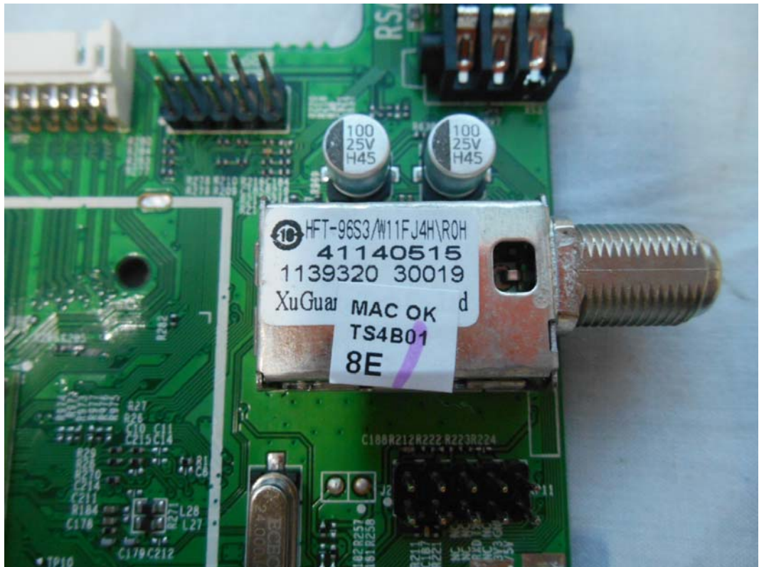
FIGURE 9 LED LCD TV (M/N: 55H4G) TUNER ON MAIN BOARD
