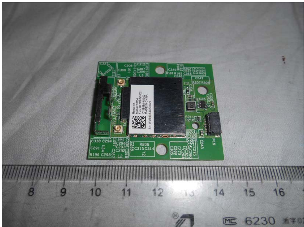
FIGURE 16 LED LCD TV (M/N: 55H4G) RF BOARD (COMPONENT SIDE)
