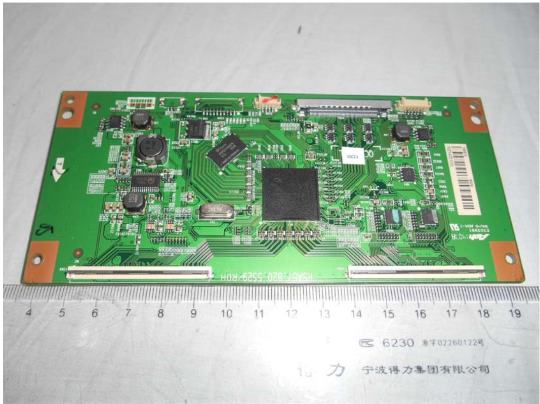
FIGURE 13 LED LCD TV (M/N: 55H4G) LCD BOARD (COMPONENT SIDE)
