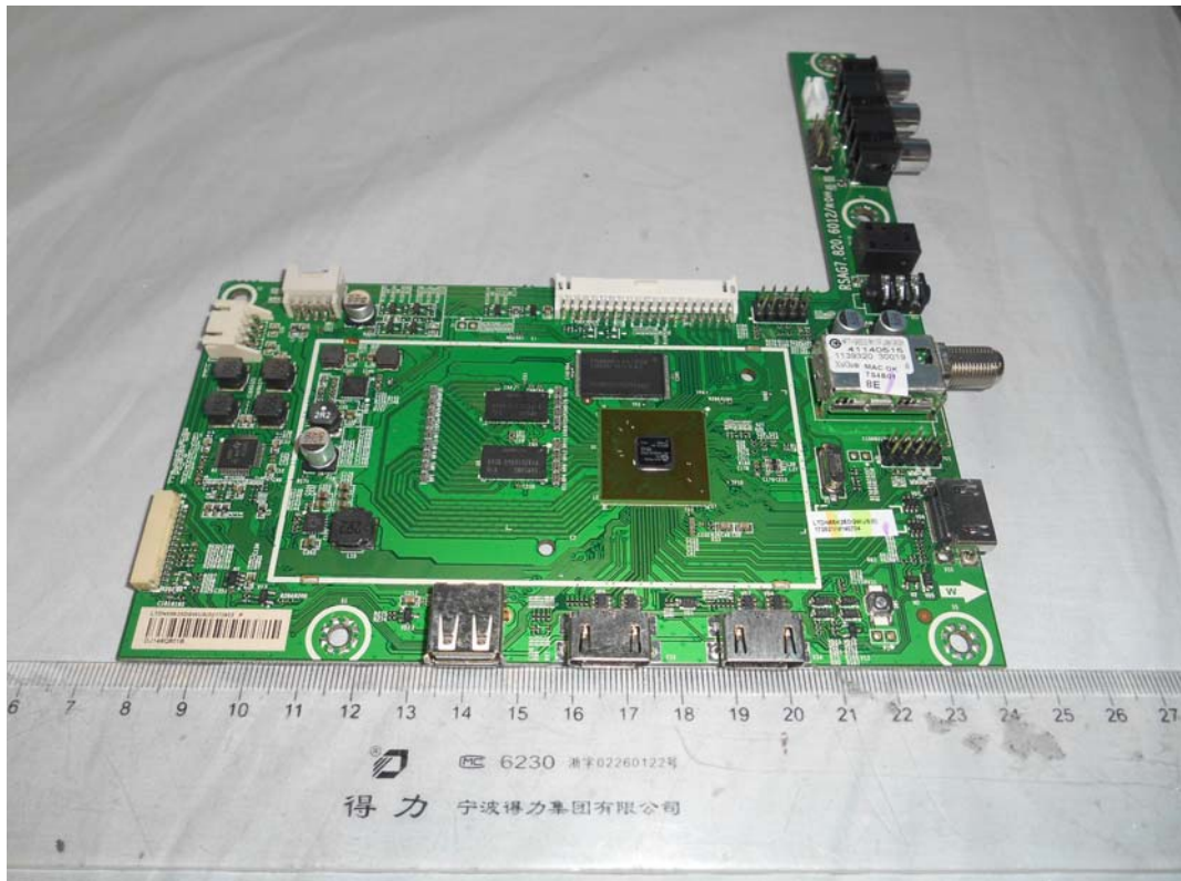
FIGURE 5 LED LCD TV (M/N: 55H4G) MAIN BOARD (COMPONENT SIDE)
