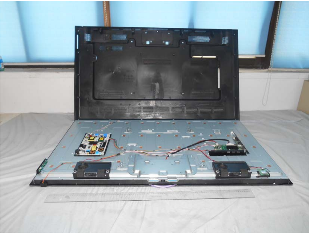
FIGURE 1 LED LCD TV (M/N: 55H4G) COVER REMOVED
