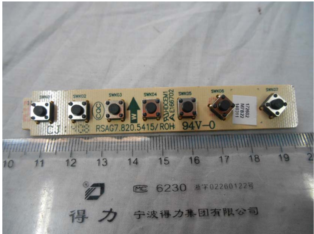
FIGURE 11 LED LCD TV (M/N: 55H4G) KEY BOARD (COMPONENT SIDE)
