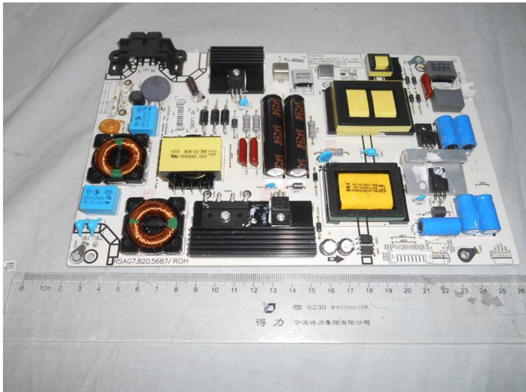
FIGURE 3 LED LCD TV (M/N: 55H4G) POWER BOARD (COMPONENT SIDE)
