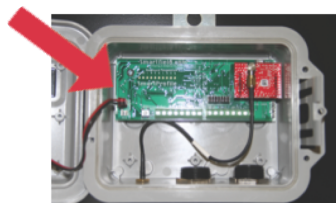
Figure 2: Showing the battery power cord plugged into the motherboard socket labeled "Battery".
