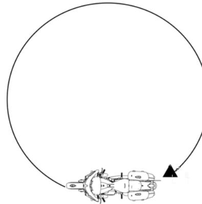
3. Once a complete circle has been driven, stop and press **PRE** to save the calibration or press **MODE** to cancel the calibration and return to the previous calibration.
