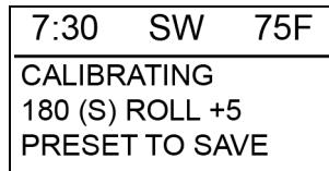
2. Drive the motorcycle at 5 mph (8km/h) in a clockwise circle keeping the motorcycle as upright as possible. Excessive tilting to the left or right will affect compass calibration.
