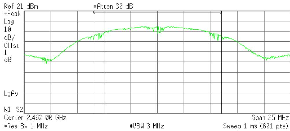
**Channel Power****13.67 dBm /12.0000 MHz****Power Spectral Density****-57.12 dBm/Hz**
