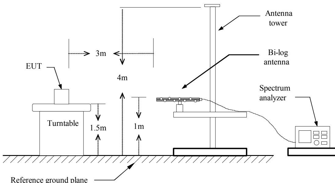
**Above 1 GHz**
