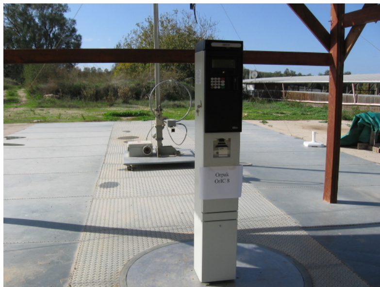
Figure 7. Radiated Emission Test Setup (9 kHz – 30 MHz)
