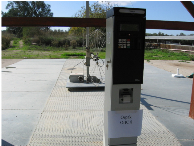
Figure 8. Radiated Emission Test Setup (30 – 1000 MHz)
