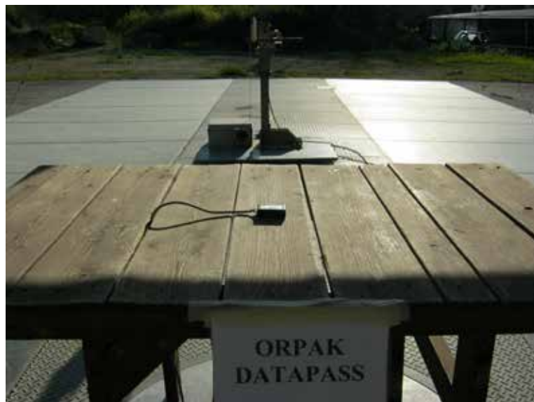
Figure 2. Radiated Emission Test Setup
