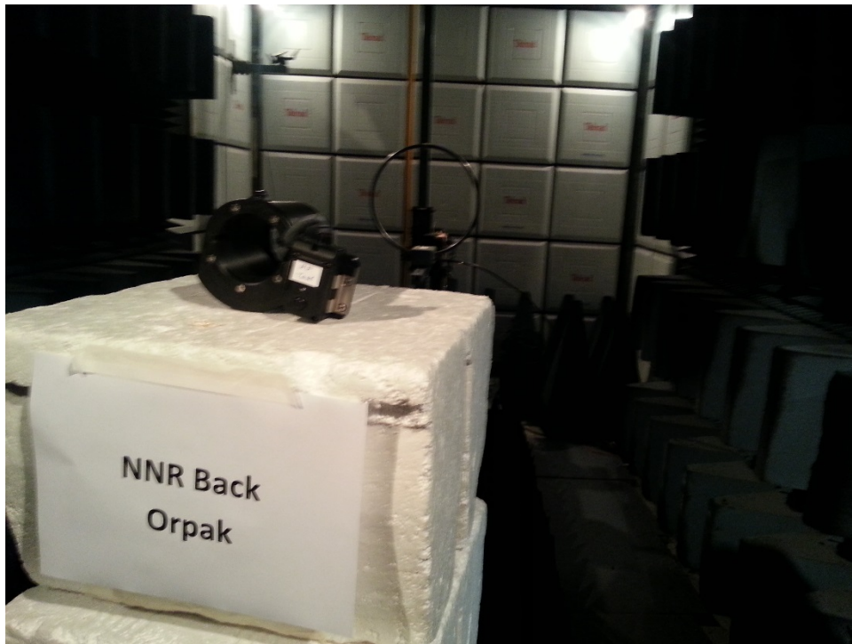
Figure 1. Fundamental and Radiated Emission Test Setup
