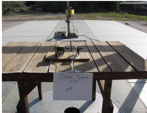
Figure 2. Radiated Emission Test Setup
