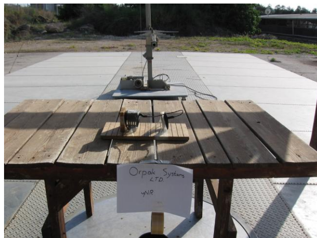
Figure 5. Radiated Emission Test Setup
