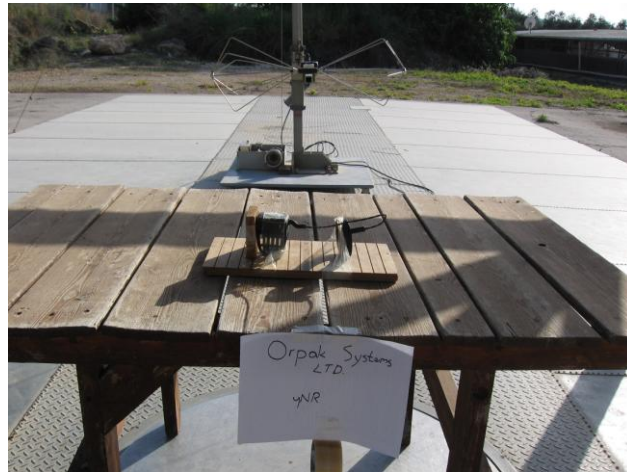
Figure 4. Radiated Emission Test Setup
