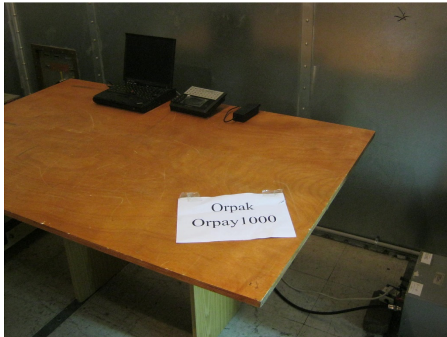
Figure 2. Conducted Emission from AC Mains Test Setup
