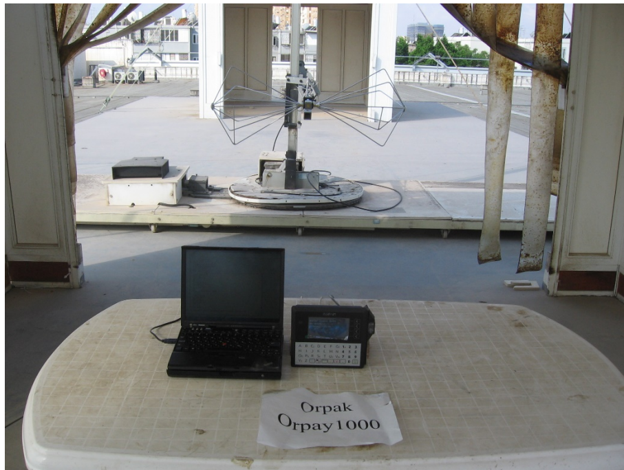
Figure 4. Radiated Emission Test
