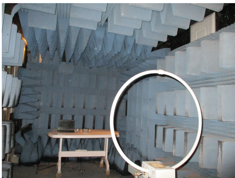
Figure 3. Radiated Emission Test Setup, 0.009-30MHz
