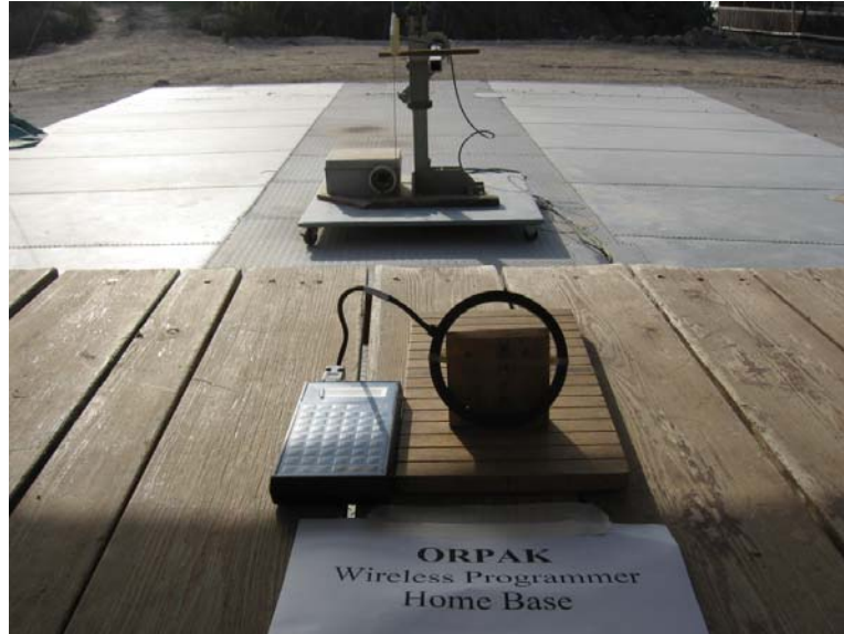
Figure 4. Radiated Emission Test- 30 MHz – 25 GHz
