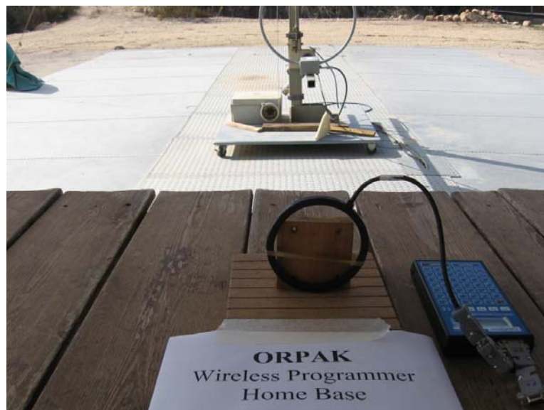
Figure 3. Radiated Emission Test 80 mm Antenna
