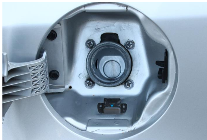
Figure 2-3 - Position 1: NanOpass Installed on the Bottom of the Fuel Compartment
