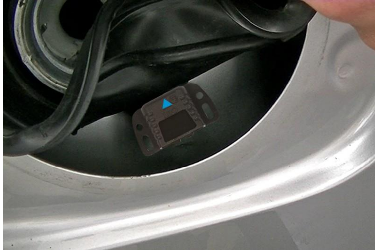
Figure 2-6 - Position 4: NanOpass Installed Behind the Rubber Gasket
