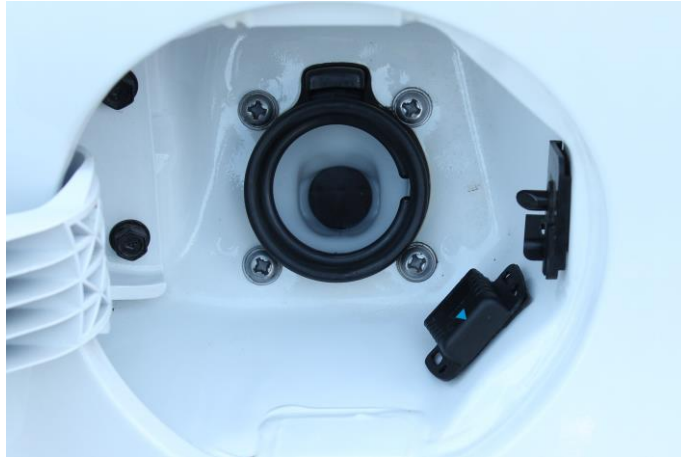
Figure 2-4 - Position 2: NanOpass Installed in a Corner at the Side of the Fuel Compartment
