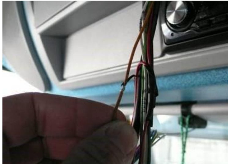
Figure 3-23 - Connecting DataPass Harness to Tachograph Wiring
