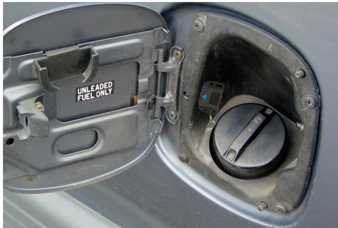
Figure 2-5 - Position 3: NanOpass Installed at the Side of the Fuel Compartment
