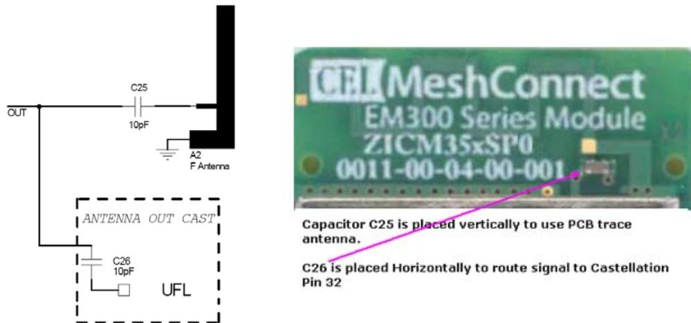
Given that the only change to the module from the existing module is the orientation of a capacitor, the transmitter is identical and the frequency of operation is exactly the same as the existing certified module. RF testing at a certified lab has been completed and has verified that the RF performance has not degraded when connected to the external antennas.
