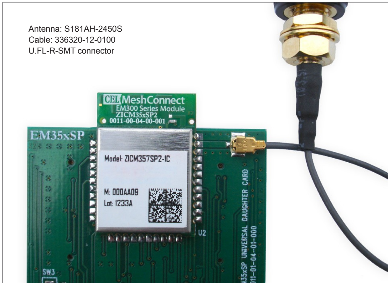
Figure 4. Implementation using connector, cable and external antenna
