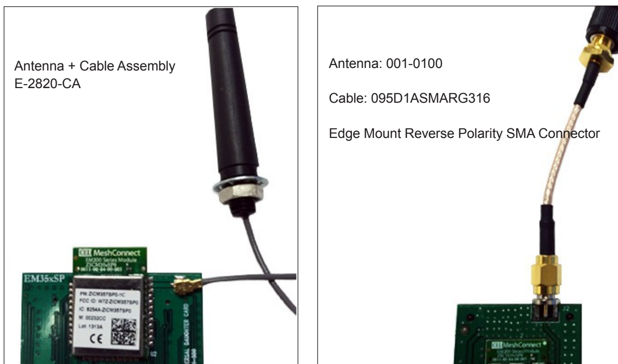
Figure 3. Implementation using connector, cable and external antenna
