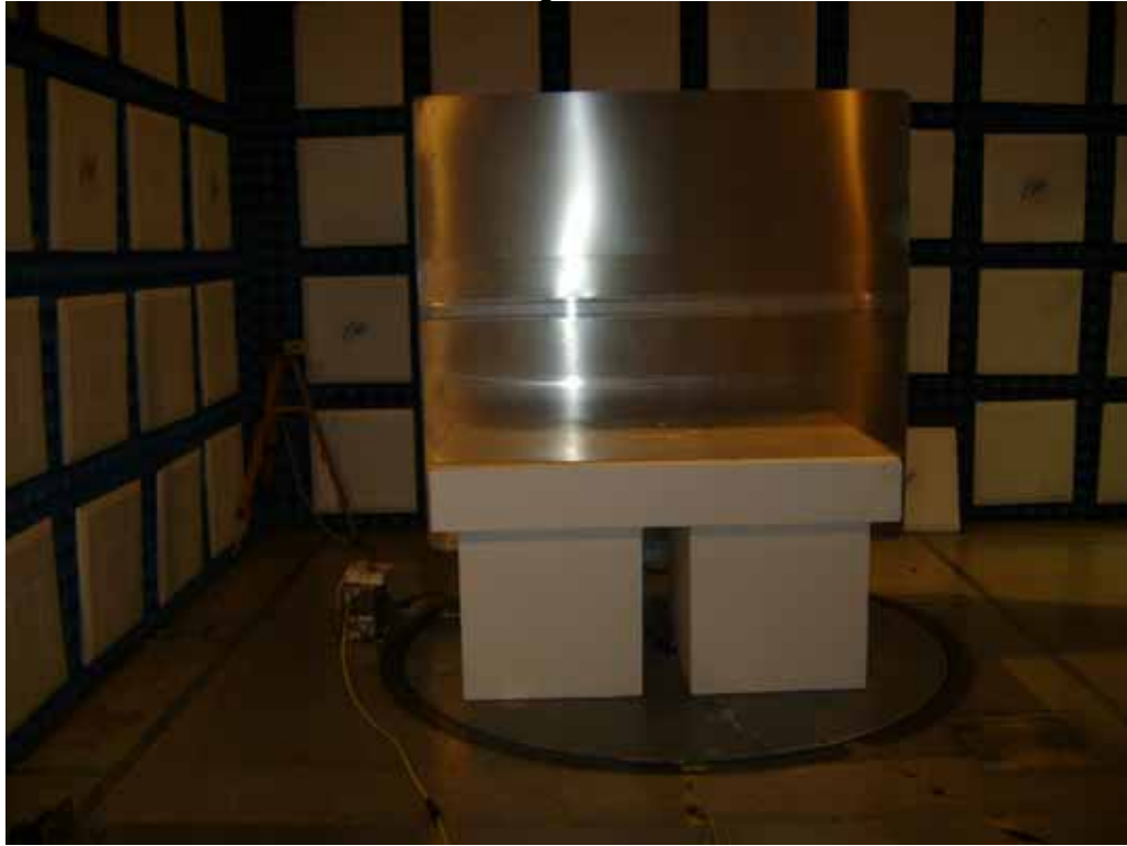
Test Setup for Conducted Emissions
