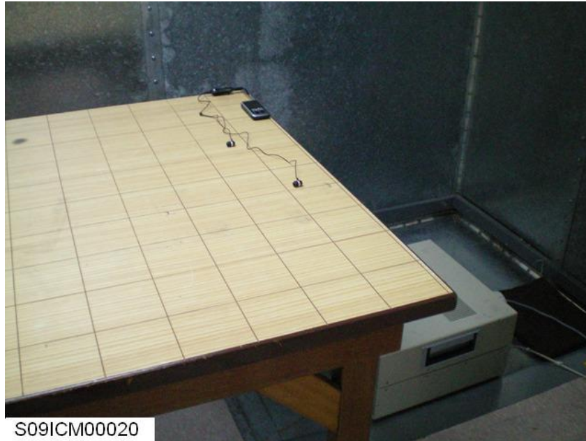
Conducted Emissions Test Setup (Front View)
