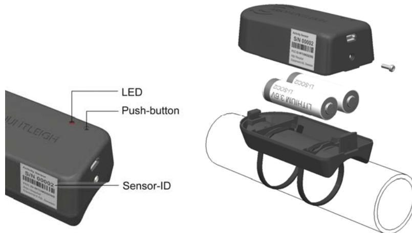
Insert the two supplied batteries, observe the polarity indicated on the PCB.
