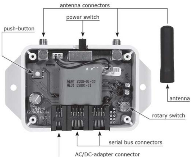
Note: Serial bus is not used for REPO+
