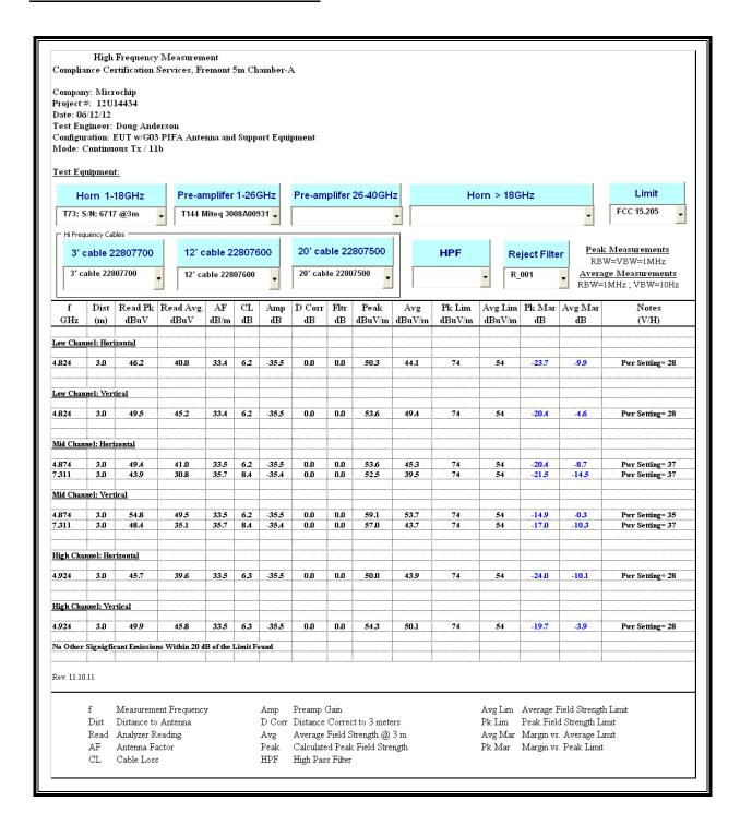
TX ABOVE 1 GHz FOR 802.11g MODE (PIFA ANTENNA)
