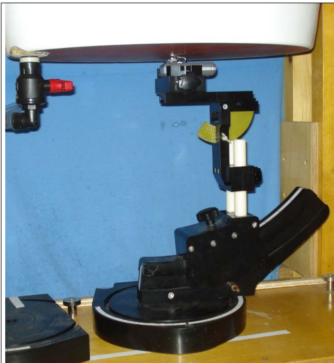
Body-worn SAR Configuration Test Setup with Belt-Clip
