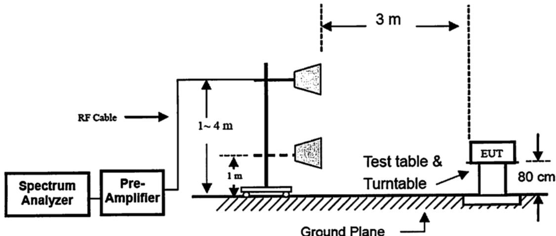
**SETUP DRAWING, SETUP DRAWING – RADIATED TX SPURIOUS EMISSIONS (< 1 GHZ)**
