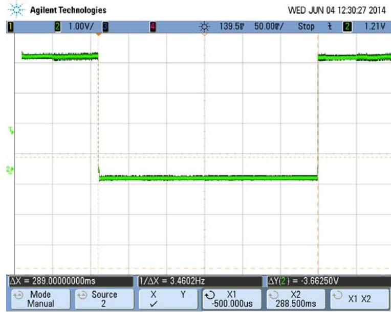
Figure 3 Time of occupancy during maximal length payload
