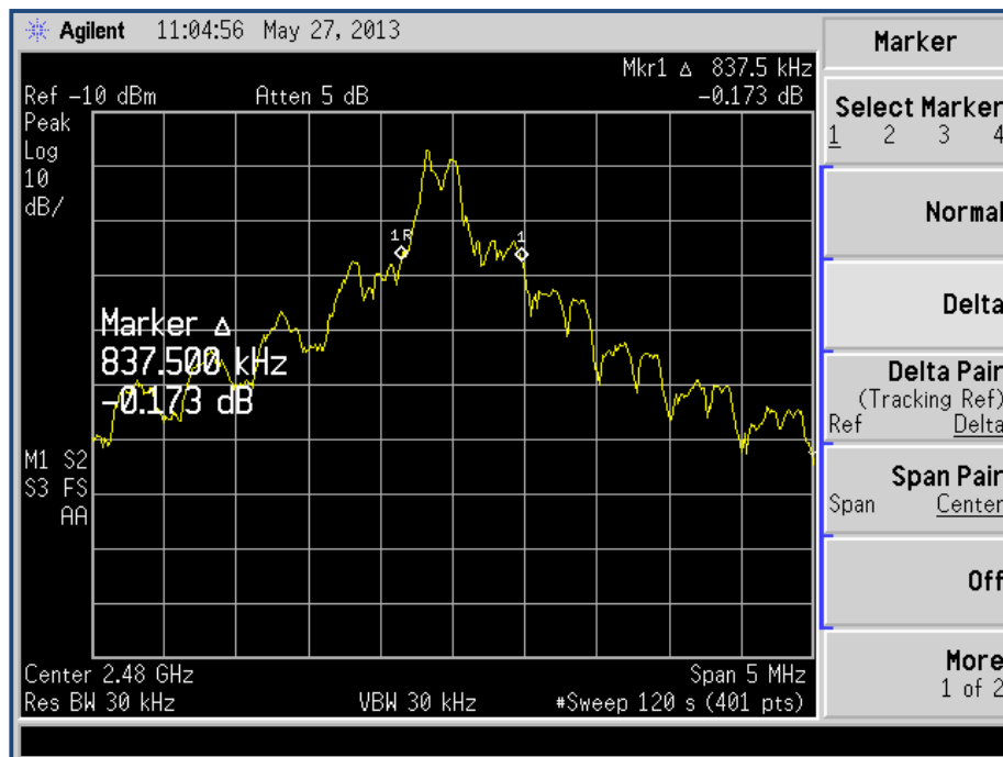
FIGURE 8 - OCCUPIED BANDWIDTH 20DB HIGH CHANNEL
