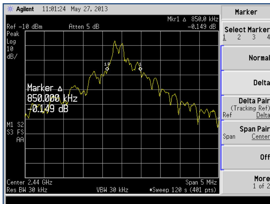
FIGURE 6 - OCCUPIED BANDWIDTH 20DB MID CHANNEL
