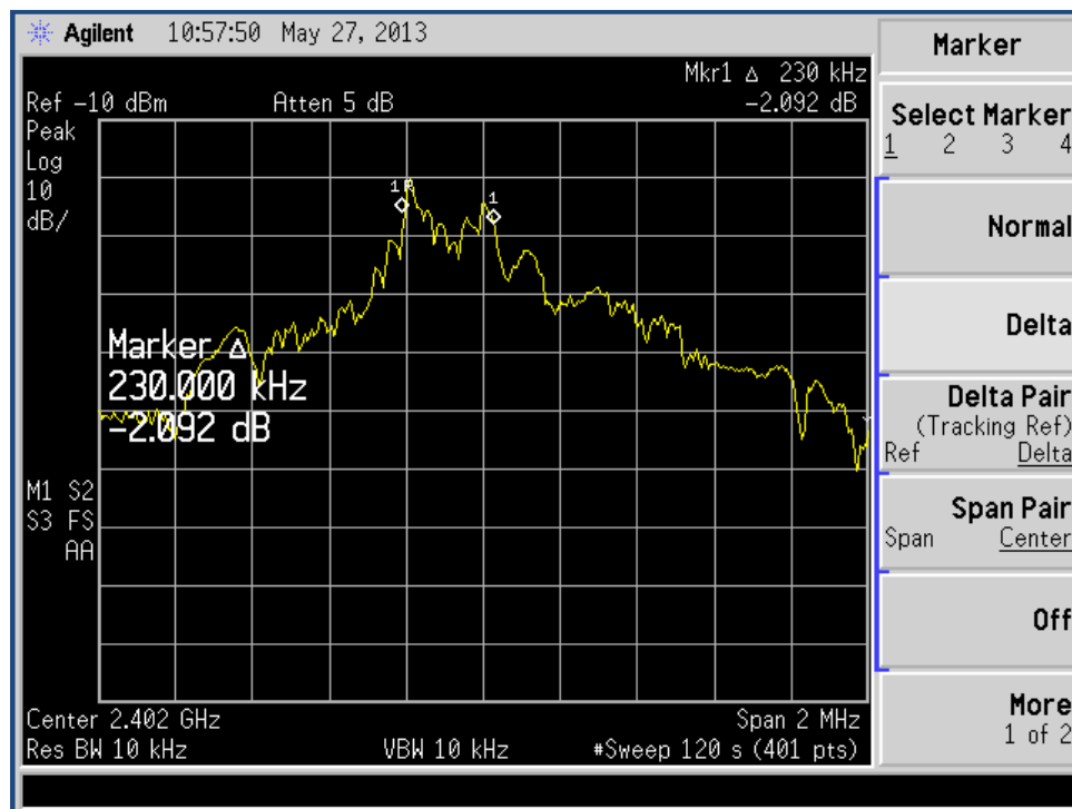
FIGURE 5 - OCCUPIED BANDWIDTH 6DB LOW CHANNEL
