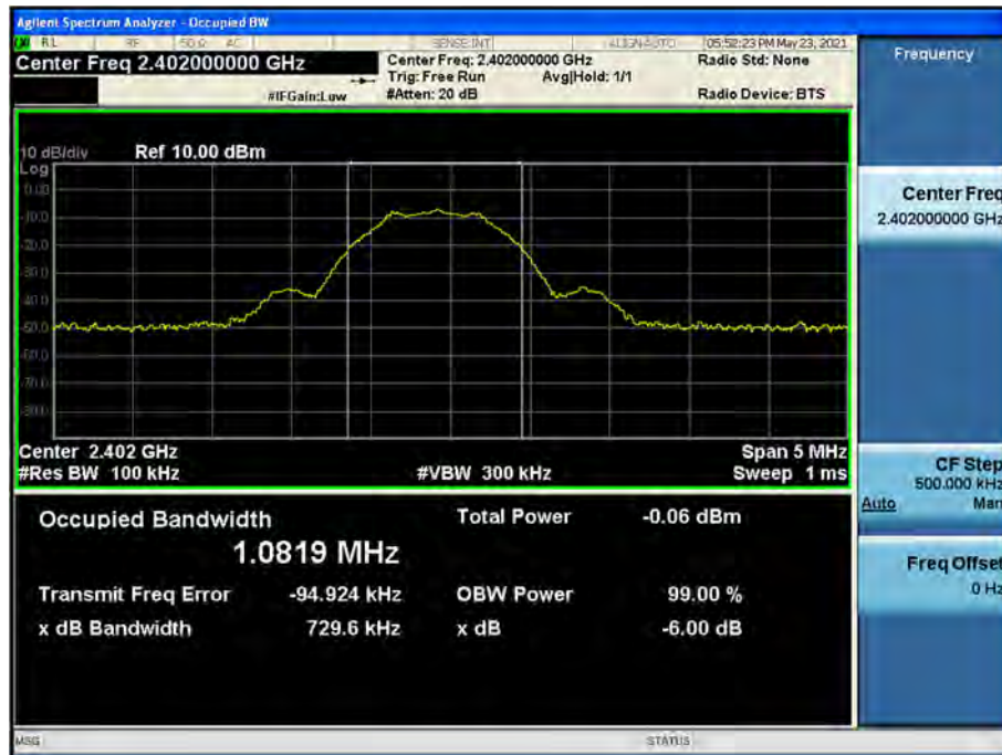
6 dB Bandwidth plot (Low-CH 0)
