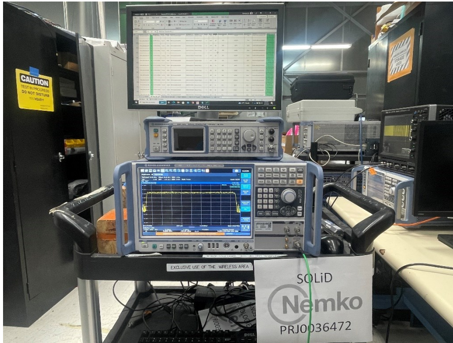
Figure 8 – Test setup (spectrum analyzer measurements)
