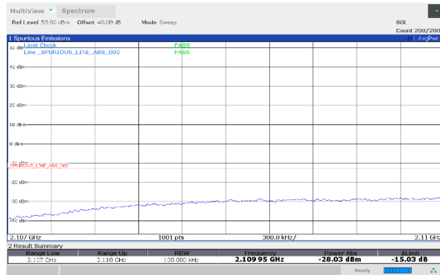
Low band edge, 2 signals, total level = 0.5 dB less than AGC threshold
